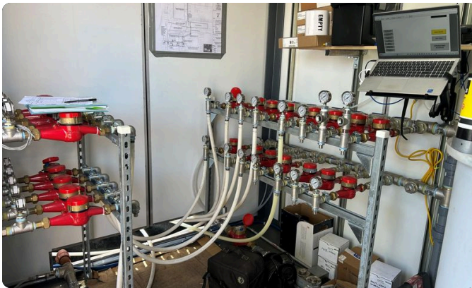
Recirculation manifolds inside the skid, and the heater and manifold skid during shop assembly and testing.
