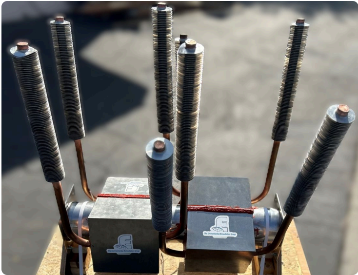
HETR™ heater assembly during fabrication.
